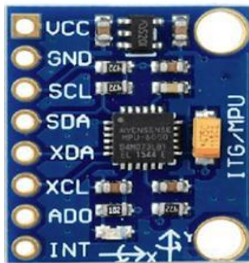
Gambar 3. Sensor Gyro Accelerometer MPU6500
